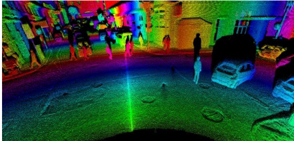
Figure 1 - Processed point cloud from LiDAR technology. The colors represent the distance from the surrounding objects. [3]
