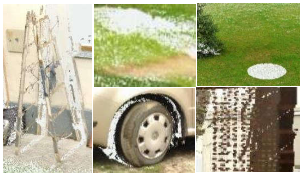
Figure 2 – Typical artifacts of raw scanner data. Top Row: Low sampling density due to gracing sensor views, Holes due to sensor restrictions, noise. Bottom Row: low sampling density at delicate surface details and outliers Left: holes due to critical reflectance properties.
