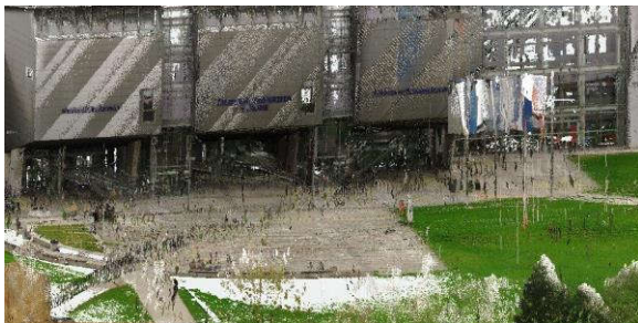
Figure 3 – Typical artifacts of raw scanner data
