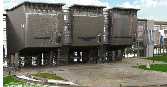
Figure 4 – Scan after application of filters, point reduction and cleansing from other scanning irregularities
